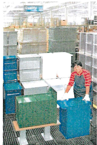
Final inspection of pedestal drop boxes
